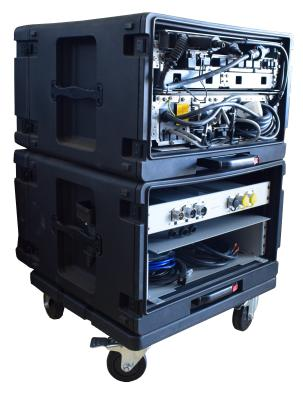
The Tactical Cube is a transportable solution, realised by Athonet, a Hewlett Packard Enterprise acquisition, that includes a radio (RAN) and mobile core. The mobile core is hosted on off-the-shelf servers or on Athonet EX-BOX server providing and the radio acts as a base transceiver station with IP65 protection. Two servers can be added for high availability and redundancy.
